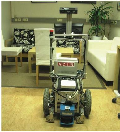
Fig. 3. Mobile robot with the stereo camera mounted on top
