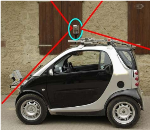
Fig. 7. The vehicle used in our experiments equipped with the omnidirectional camera (in the circle). The vertical field of view is indicated by the lines.
